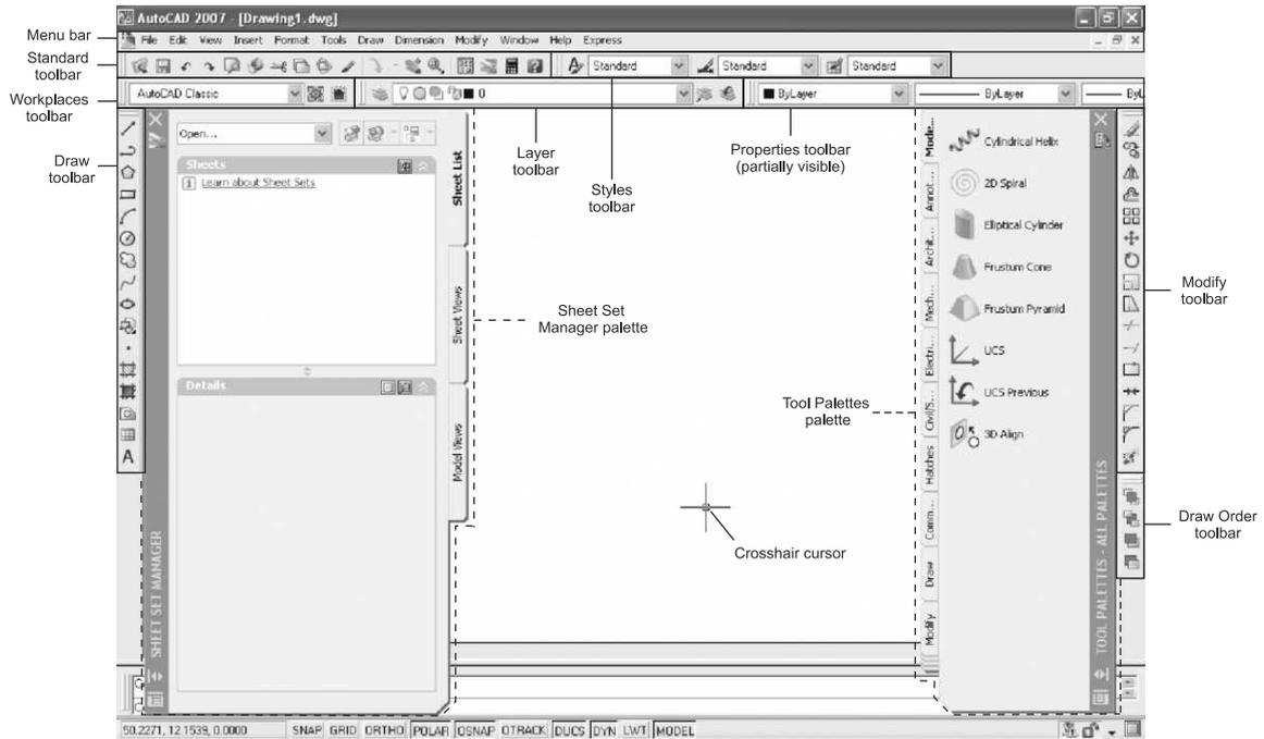
Fig. 22.10(a) AutoCAD Window\* with Sheet Set Manager palette and Tool Palettes palette
