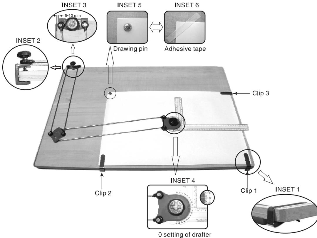
**Fig. 1.21** Clamping the drawing sheet and drafter
