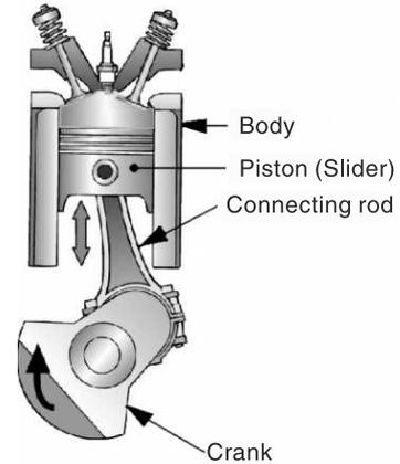
**Illustration 7.2** Automobile engine—An example of slider crank mechanism
