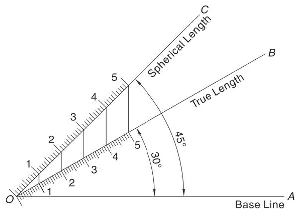
Fig. 18.23 Spherical Scale
