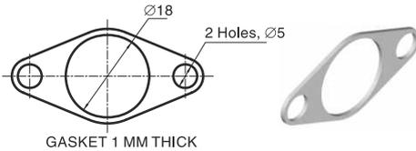
(a) Use of note 'GASKET 1 MM THICK' provides an idea about the thickness of the flat gasket.
