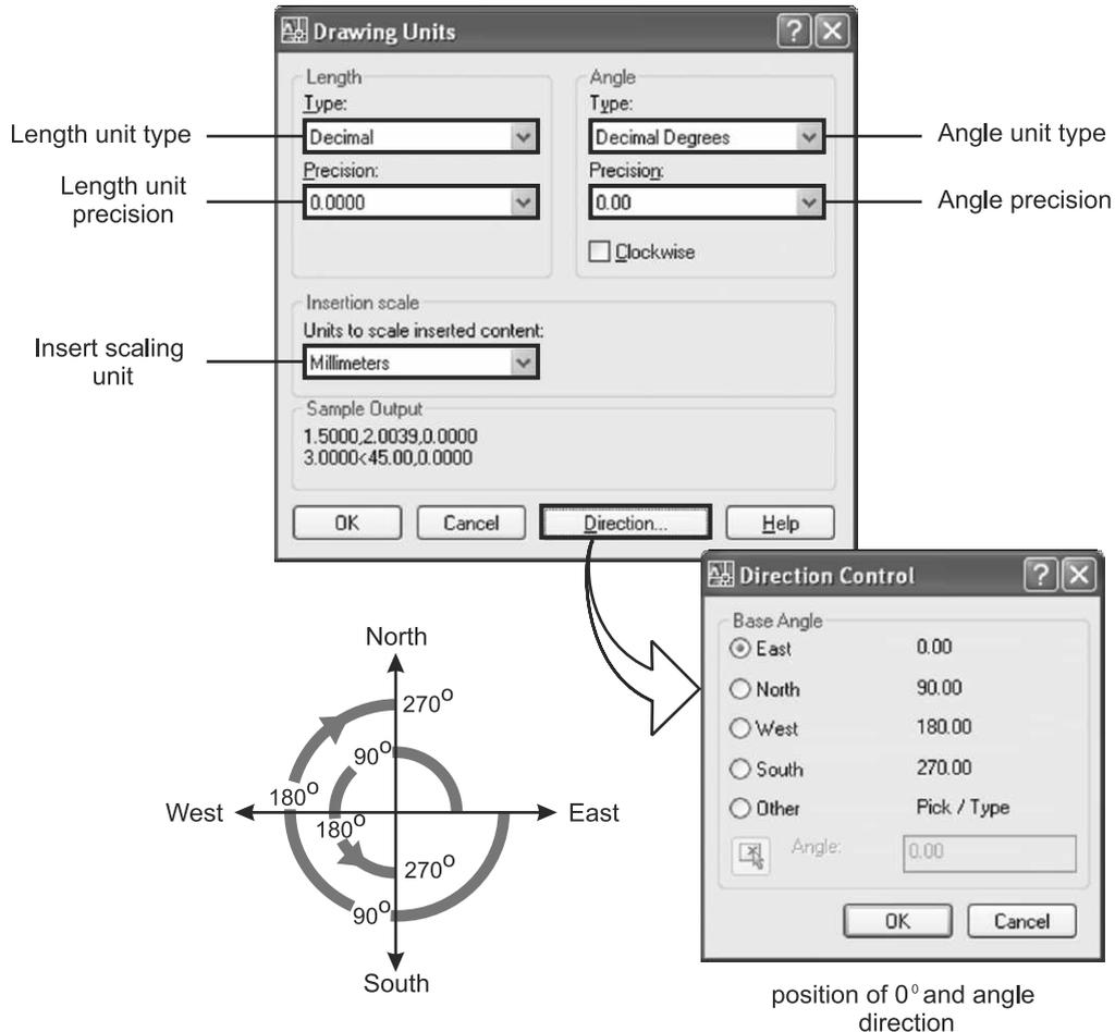
Fig. 22.13 Drawing Units Dialog Box with Direction Control Option
