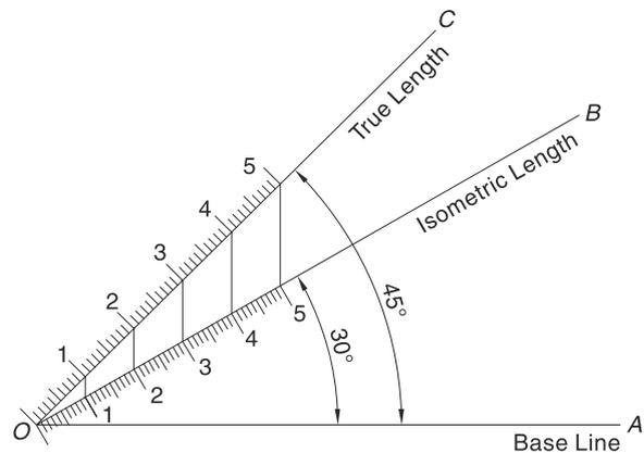
Fig. 18.4 Isometric Scale
