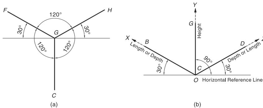
Fig. 18.3 Isometric Axes and Isometric Lines
