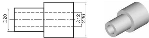
(b) Use of centerline and ' $\phi$ ' symbol provide an idea about the cylindrical object.
