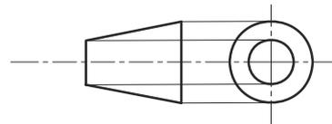
**Fig. 9.2** First Angle Method of Projection
