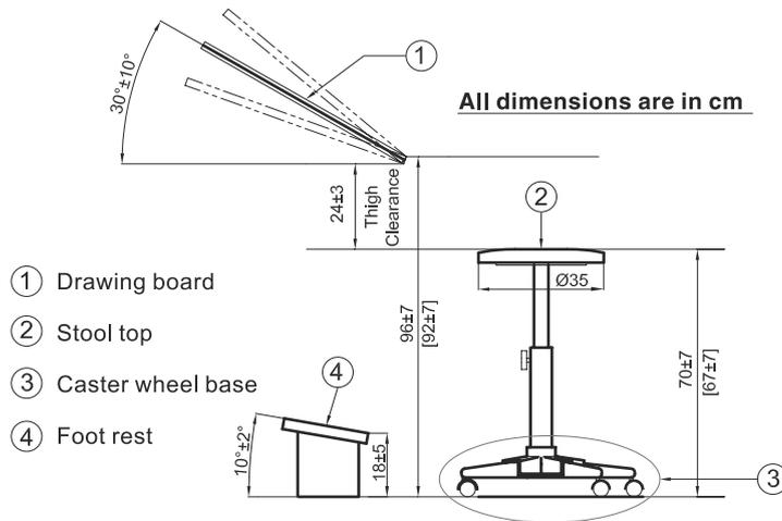
Fig. 1.29 Ergonomic drawing set-up
