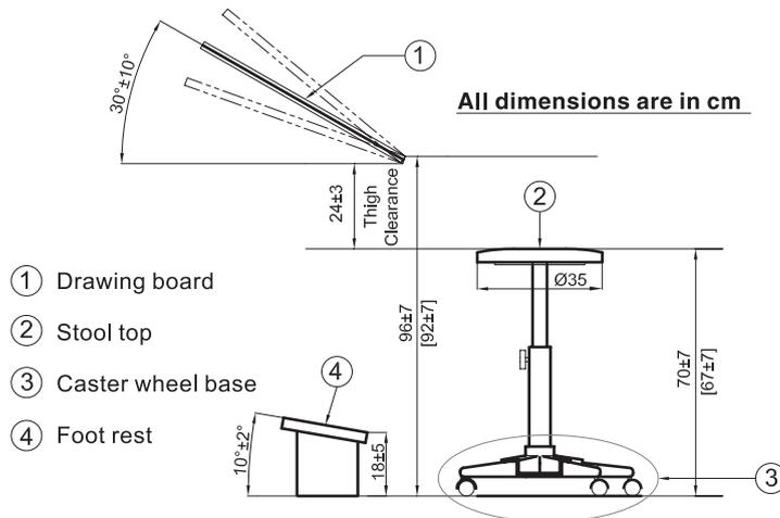
Fig. 1.29 Ergonomic drawing set-up
